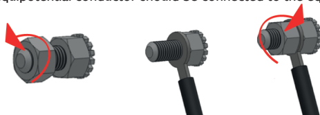
Figure 5. Connection of the device to an installation equalizing electrical potentials.
