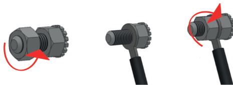
Figure 7. Connecting the unit to an electrical equalizing system
